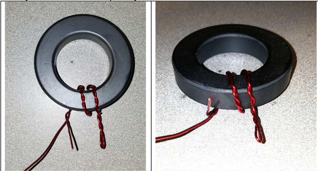
Keep winding the long secondary wire (keep track of turns).
