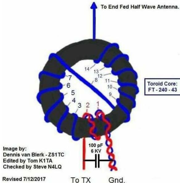
Wind two turns of the double wire section on the toroid as shown
