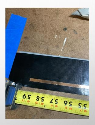
Step 2: Layout the copper tape according to precise dimensions.
