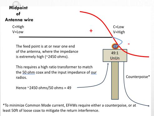
\*\*\*\* Note: this is a  $\lambda/2$  radiator, hence the top bend of the physical antenna is approx. the center point of the antenna.
