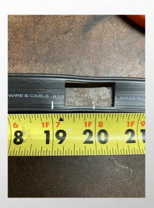
Step 3: Cut the 1" stub gap, and reinforce the ladder line gap with tape to keep it from Sagging.
