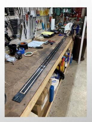
Step 4: Use clothes pins or magnets to hold the feedline in place for tuning adjustment
